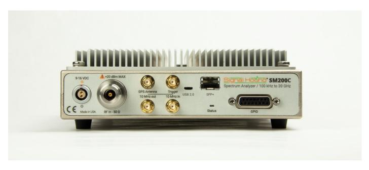
The SM200C is a high-performance spectrum analyzer and monitoring receiver with a 10 Gigabit Ethernet SFP+ port, which enables the SM200C to communicate with a PC over long distances using a fiber optic cable. Tuning from 100 kHz to 20GHz, the analyzer has 160 MHz of instantaneous streaming bandwidth (IBW), 110 dB of dynamic range, 1THz/sec sweep speed at 30kHz RBW (using Nuttall windowing), and phase noise performance that rivals even the most expensive spectrum analyzers on the market.
